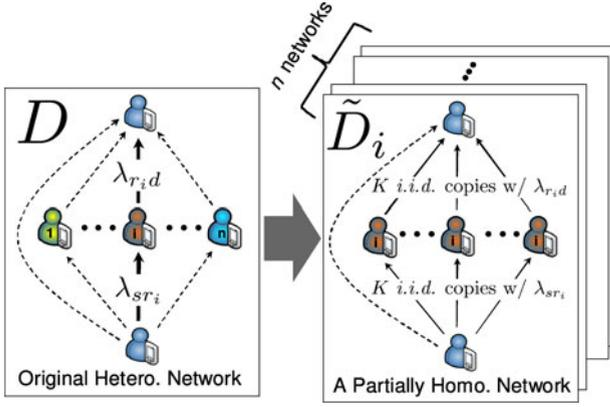
Fig. 3. Decomposition of a heterogeneous network into  $n$  partially homogeneous networks  $\mathfrak{N}_i$ .  $K$  two-hop relay paths in  $\mathfrak{N}_i$  are *i.i.d.* copies of the two-hop relay path via relay node  $r_i$  in the original heterogeneous network.
