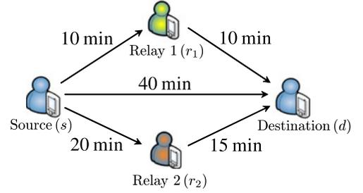
Fig. 4. An example scenario for a source-destination pair with two possible relay nodes. The average inter-contact time for each node pair is shown along the arrow.
